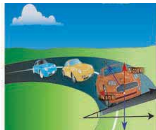
Figure 3.44 Outer edge of the road is slightly raised to avoid skidding
